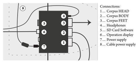
Figure 3-8: Wiring diagram of the control unit in the technical compartment
